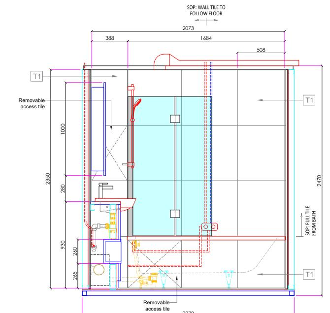
• WALLS WILL BE STRONG ENOUGH TO SUPPORT AN IMPOSED LOAD OF 1.5KN/M2. THE LAYOUT MEETS THE CLEAR ACCESS ZONES REQUIREMENT IN M4(2) DIAGRAMS 2.5 & 2.7.
